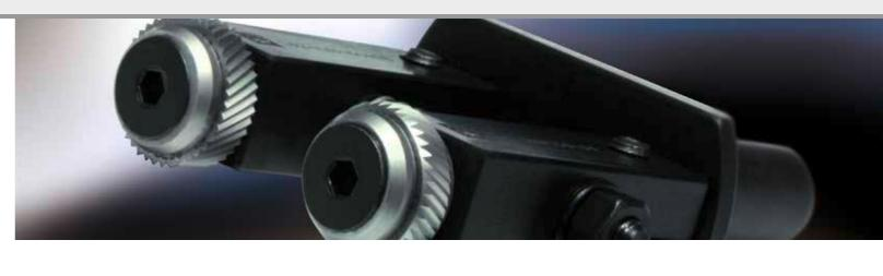
The zeus® RD2 series 161/162 allows for a fine machining. Due to the special tool design with two knurl holders, the lateral pressure exerted on work piece and machine is minimal. The series is therefore especially suitable for form knurling small and delicate parts. Several versions are available for different applications and machine types. Where work space is limited and tiny work piece diameters have to be knurled, this tool range should be the first choice!
