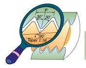
Conical pipe thread inserts are onesided and may be used for both External and Internal threading.
