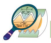
Conical pipe thread inserts are onesided and may be used for both External and Internal threading.
