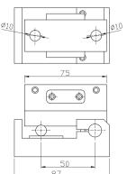
This fine precision-made unit dresses grinding wheels to any angle from 0°-60° degrees with new smoothness and accuracy.
